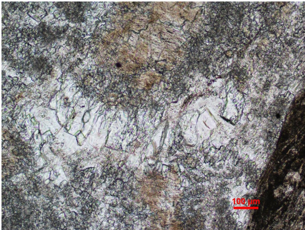
Sample CD-1. Foliated sericite-muscovite in mylonitic shear cutting remnant carbonate vein. Top-plane light; Bottom- crossed polarizers.
