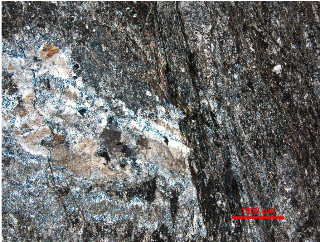
Sample CD-1. Remnant carbonate veins disrupted by mylonitic shear. Top- plane light; Bottom- crossed polarizers.
