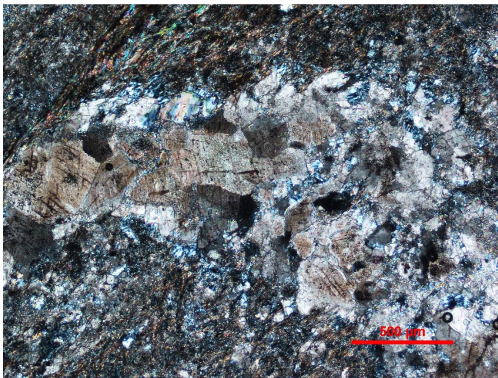
Sample CD-1. Different stages of carbonate in relict carbonate vein. Top- plane light; Bottom- crossed polarizers.
