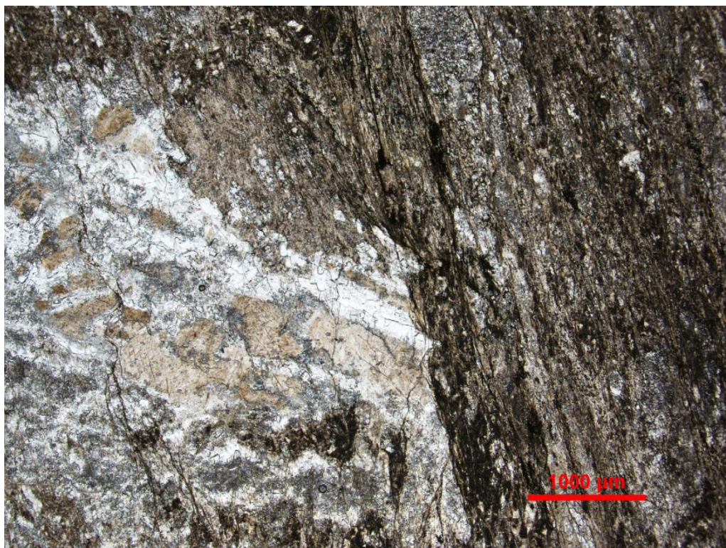
Sample CD-1. Mylonitic shears in carbonate. Top- plane light; Bottom- crossed polarizers.
