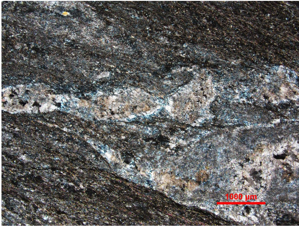
Sample CD-1. Sheared and boudinaged carbonate veins. Top- plane light; Bottom- crossed polarizers.
