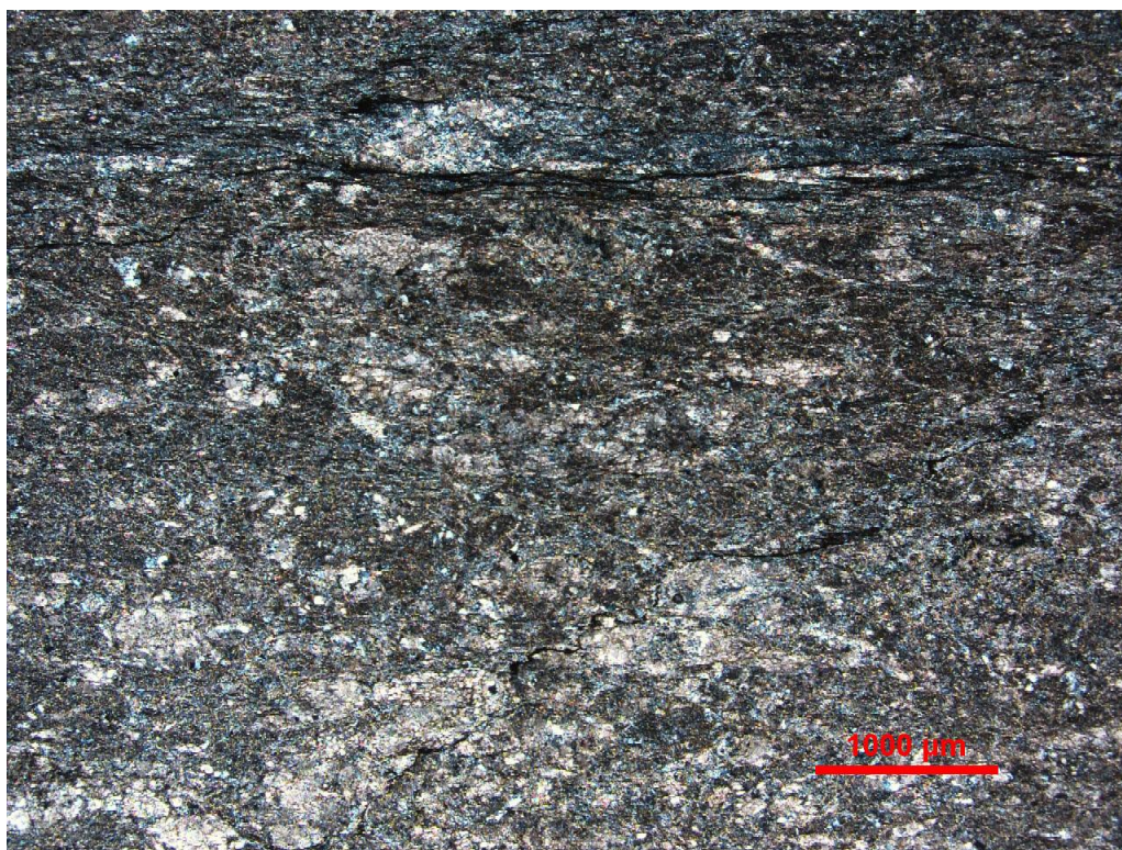
Sample CD-1. Mylonitic shears in carbonate. Top- plane light; Bottom- crossed polarizers.
