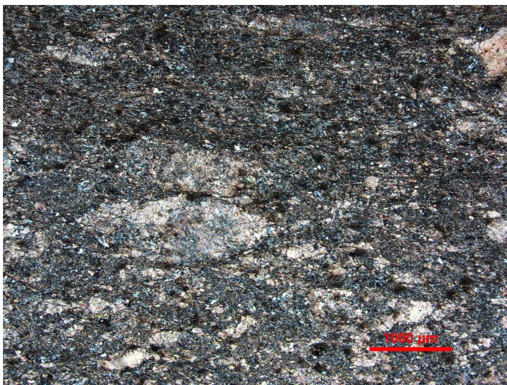
Sample CD-1. Sheared and foliated carbonate with relict carbonate lenses. Top- plane light; Bottom- crossed polarizers.
