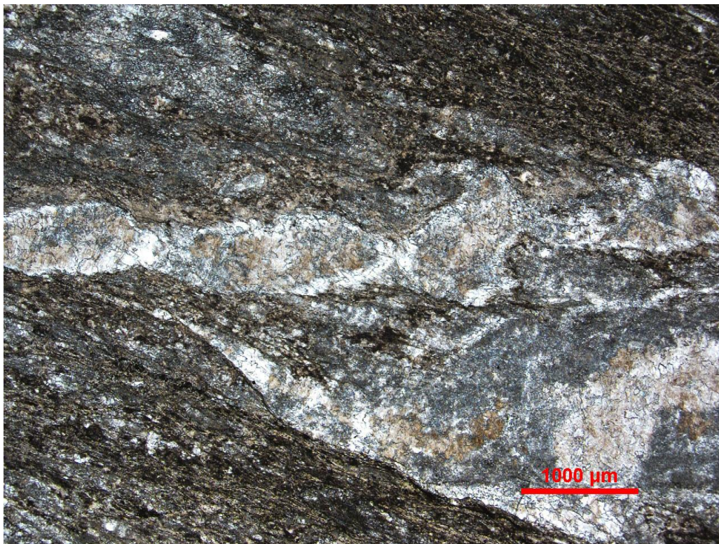
Sample CD-1. Remnant carbonate veins disrupted by mylonitic shear. Top- plane light; Bottom- crossed polarizers.
